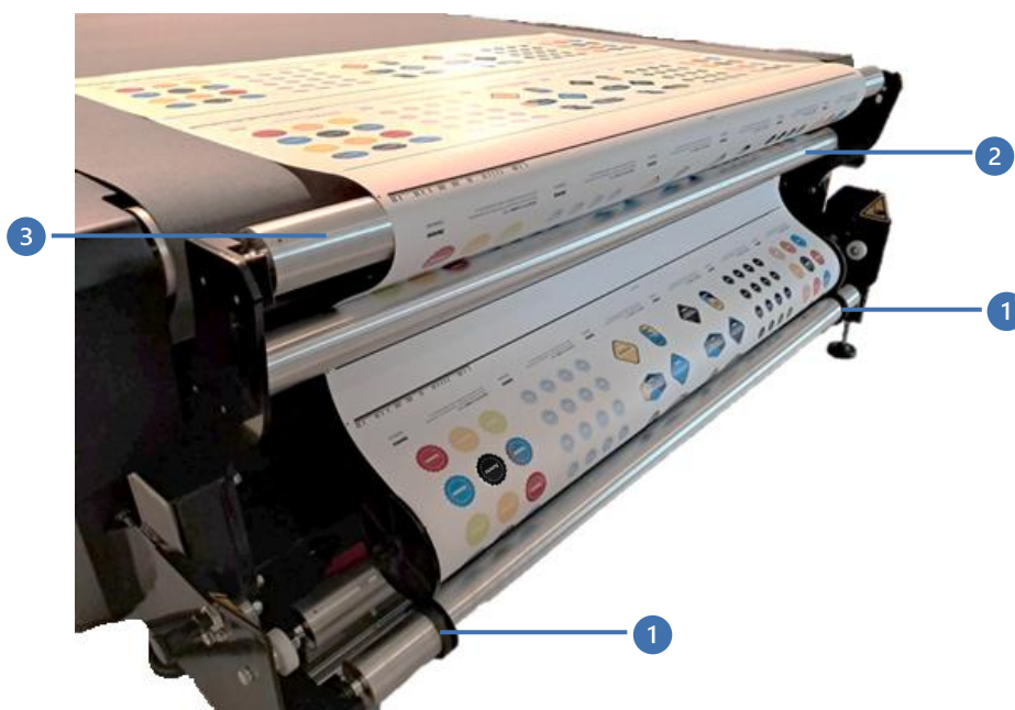
FIG 2-1 LOADING MEDIA < 25KG ON LOWER SUPPORT ROLLS
