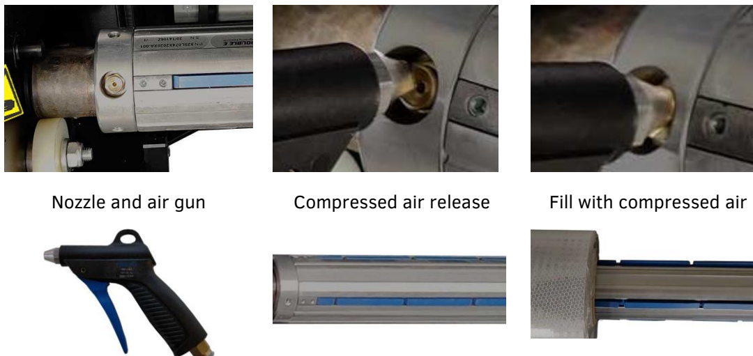
FIG 2-2 DETAILS BLUE PNEUMATIC EXPANSION SHAFT
