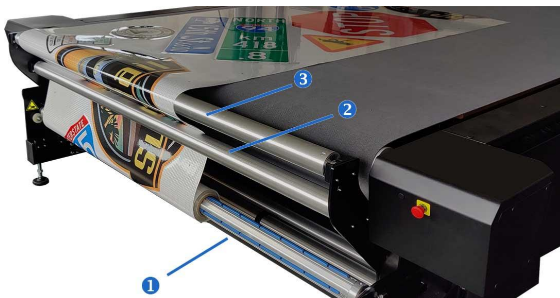
FIG 2-5 LOADING HEAVY MEDIA WITH THE PES
