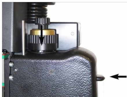
FIG 2-22 INSTALL THE UPPER PART OF THE V-CUT TOOL
