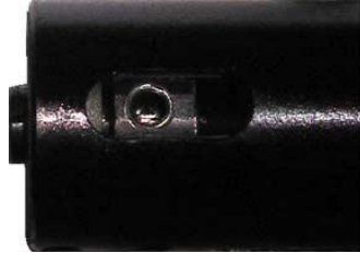
FIG 1-31 KNIFE HOLDER SHAFT – SETSCREW REMOVED FROM EOT
