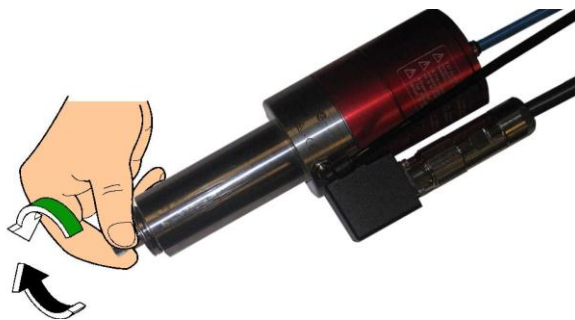
FIG 4-13 RE-INSTALL THE COLLET FROM THE MILLER
