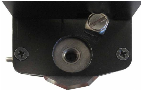
FIG 2-28 PLACE NEW KNIFE IN ROTARY MODULE
