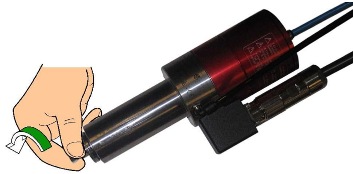
FIG 4-11 REMOVING COLLET FROM THE MILLER
