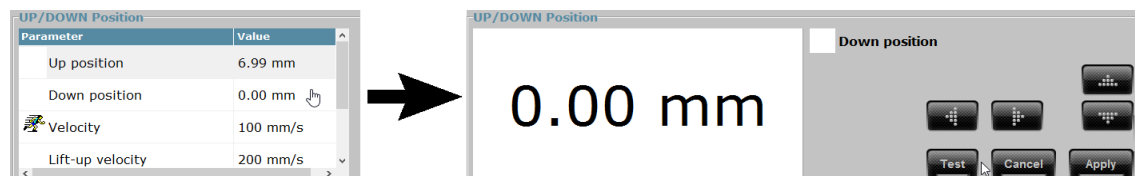
FIG 2-38 CHECKING THE CUTTING DEPTH
