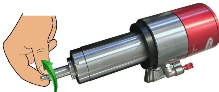
FIG 4-15 REMOVING COLLET FROM THE MILLER
