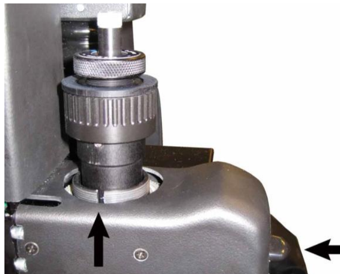
FIG 2-13 INSERT THE KISS CUTTING TOOL
