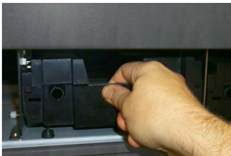
FIG 1-16 REMOVING A CASSETTE
