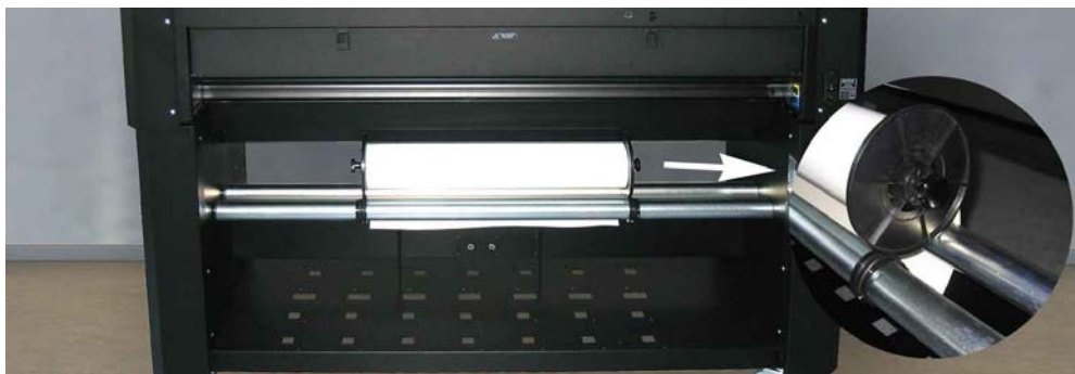
FIG 1-11 POSITION OF THE SUPPLY ROLL ON THE DC4SX
