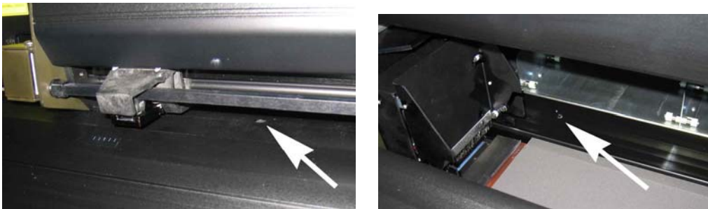
FIG 5-2 POSITION OF THE FRONT AND REAR MEDIA SENSOR
